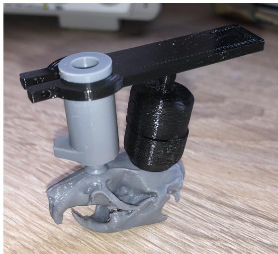
Figure 3.12: The assembled headgear with the 3D-printed components.
