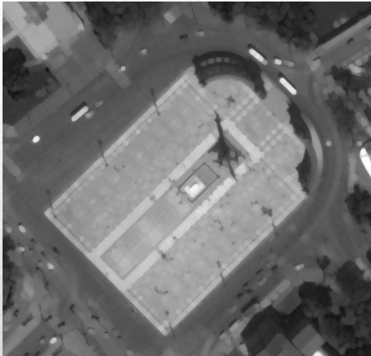
Opening & closing with 5 pixel radius STREL
