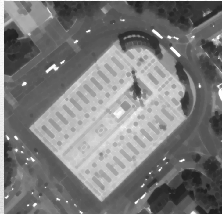
Opening & closing with 5 pixel radius STREL
